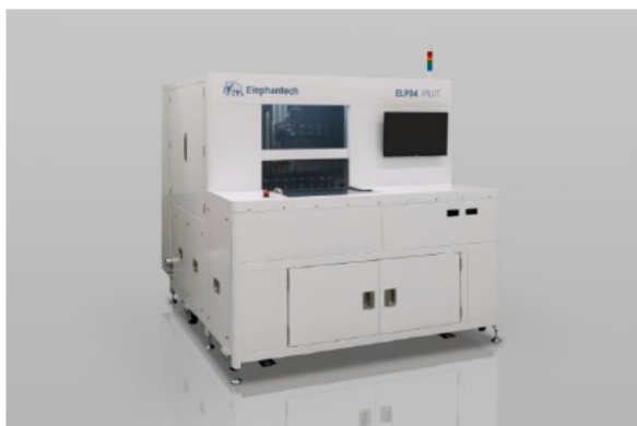
Inkjet printer for Cu nanoparticle ink
