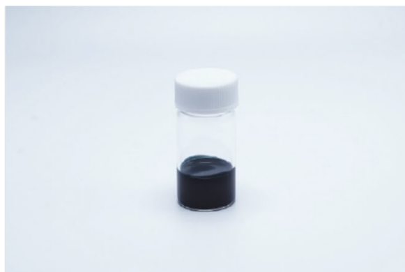
Cu nanoparticle ink for HDI microvia
