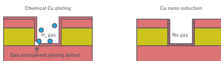
Comparison of Cu nano reduction VS electroless plating
