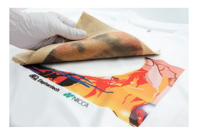
The Neochromato process jointly developed by Elephantech and NICCA CHEMICAL contributes greatly towards reducing the industry's environmental impact and has the following characteristics:
