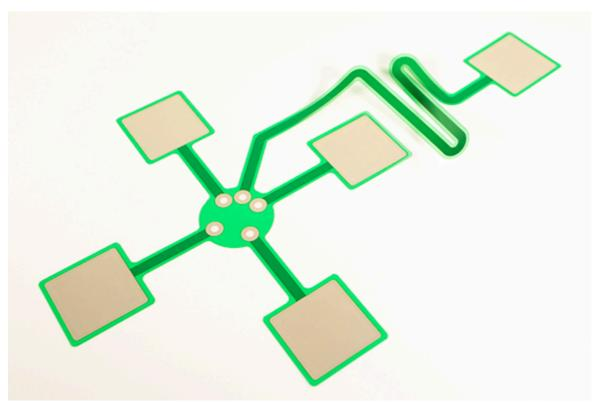
Bioelectrodes are used to detect bioelectric potentials such as ECG (electrocardiogram), EEG (electroencephalogram) or EMG (electromyogram). There are several kinds of electrodes but, especially for monitoring, the use of Ag/AgCl electrodes is well-suited as it can be used stably over long periods of time and has a low polarizing potential between the skin and the electrodes.
