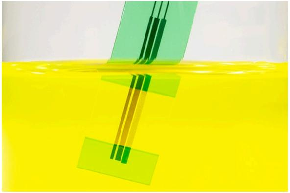
An electrochemical sensor is a sensor that can sense the state by using redox potential. It is used in environmental and water quality analyses to measure the amount of copper, arsenic, mercury and the like contained within the water. In addition to this, as the transducer part of a biosensor, it is used in blood glucose level, lactic acid, urine sugar, and glutamic acid sensors and such.
