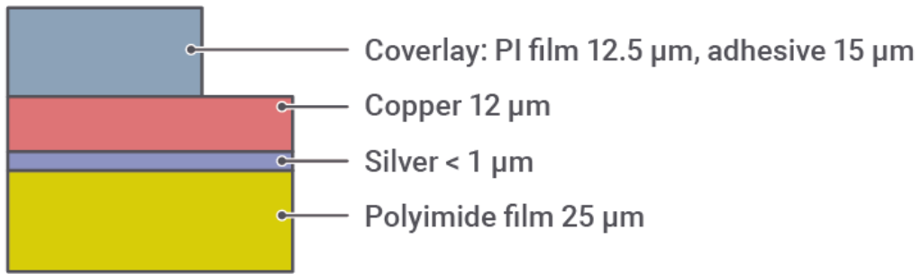
Figure The layer structure of the Thick Copper Trace P-Flex ® PI newly added to the lineup
